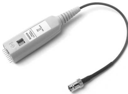
Figure 11.3. The Agilent E2622A dc-coupled, unbalanced adapter allows you to connect communications signals, such as DS3 and E3, to the oscilloscope's 50 \Omega BNC input.
