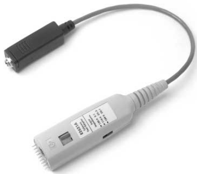
Figure 11.2. The Agilent E2621A ac-coupled, balanced adapter allows connection to differential communications signals by terminating the signal into 100, 110, or 120 \Omega .
