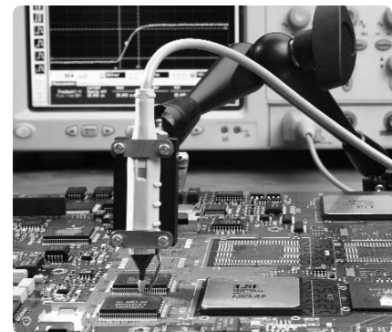
Figure 3.10. Agilent E2654A EZ-Probe Positioner option provides stable and accurate X,Y, Z probe positioning (see “EZ-Probe Positioner” in the “Probing Accessories” section of this document).
