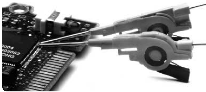
Figure 7.2. Extremely small-sized clips for probing PQFP and SOIC SMT packages.
