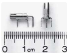
Figure 7.3. Horizontal and vertical versions of the PC board mini-probe socket make it easy to fit into your target board.
